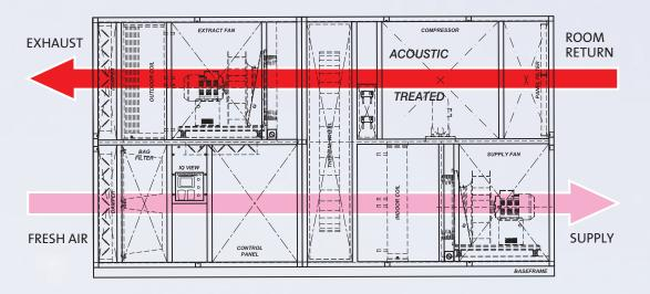
When the room is calling for a cooling requirement, and the outside fresh air temperature is lower than the room exhaust air,
