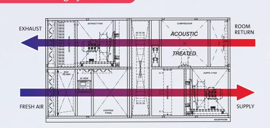
Fresh air enters the Envirofresh unit passing through the thermal wheel which transfers heat energy from the room return air before passing through the supply air coil where the high temperature refrigerant transfers its heat energy to the room supply air.
