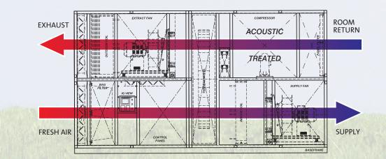
The outside fresh air enters the Envirofresh unit and passes through the thermal wheel to transfer cooling energy from the room return air. If the temperature is lower than the outside ambient air, it then passes through the supply air coil where the lower temperature refrigerant transfers its cooling energy to the supply air, further reducing the entering room air temperature.
