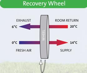
First we recover 73% of the energy from the room exhaust air to the supply air with a rotating wheel.
